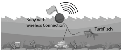
Figure 2: Integrated setup of the TurbFish and a wireless shield in a fishing float
